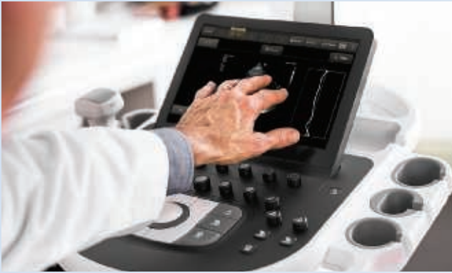
With image replication and TGCs on its tablet touchscreen, Affiniti 70 was designed to reduce reach and button pushes.
